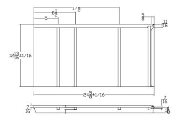
» Flashings and matching coilstock are made of .019"/.483mm 3105 H26 aluminum alloy sheet stock with a yield strength of 25 000 psi and tensile strength of 30 000 psi. Four-Way Interlocking Design
